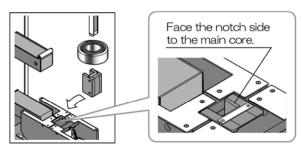
Slide the I-type core removal device so that the polishing faces of I-type core and the main core meet. Then set the temperature sensor.
