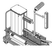
3. After placing the bearing to be heated in the I-type core removal device, install I-type core through the bore of bearing.
