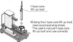
% In the case of using the I-type core which has the guide, install the guide first.
