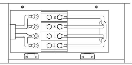
(4) Connect the terminals of the power supply cable to the terminal block.
