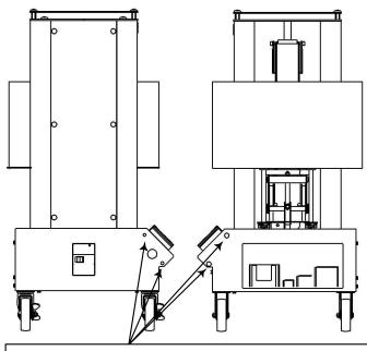
Fig 7-5 Shut the cover and tighten the four hexagonal bolts with a hexagonal wrench.
